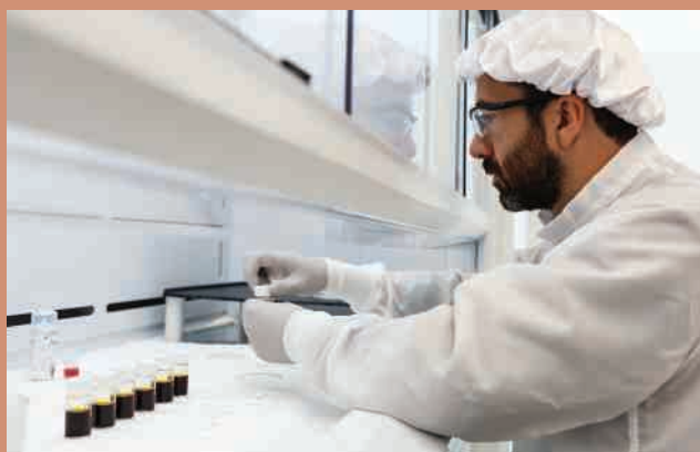
Isolation of osmium (the 2nd rarest element in Earth's crust) in the Rooney Group Clean Lab using the solvent-extraction technique
