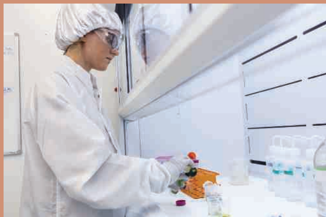
Graduate student Erica Evans isolating and purifying rhenium prior to column chromatography and analysis via mass spectrometry
