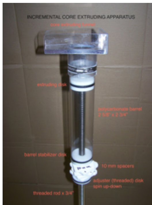
Figure 5. Example of a sediment core extrusion apparatus. 1 cm spacers are used to ensure collection of equal sediment samples. (Image courtesy of Aquatic Research Instruments)
